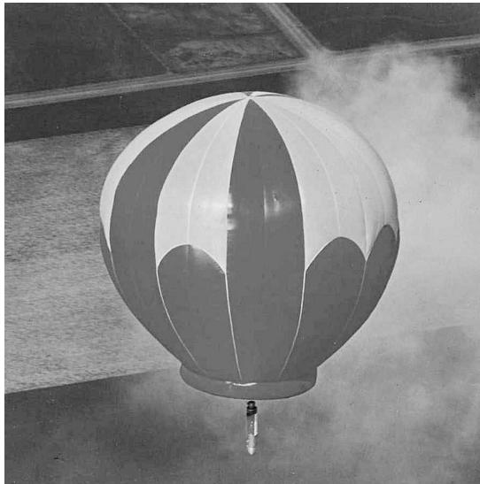
Fig. 7. Ballute fully inflated, heated & flying level. Photo Rekwin Achieve.
