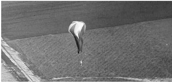
Fig. 6. Falling and inflating. Note systems canister below mouth of ballute. Photo Rekwin Achieve.
