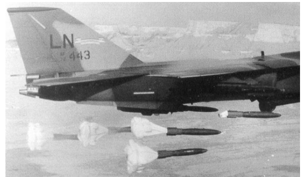
Fig. 4. Ballute inflation during munition release at high speed. Photo Irvin Aerospace.
